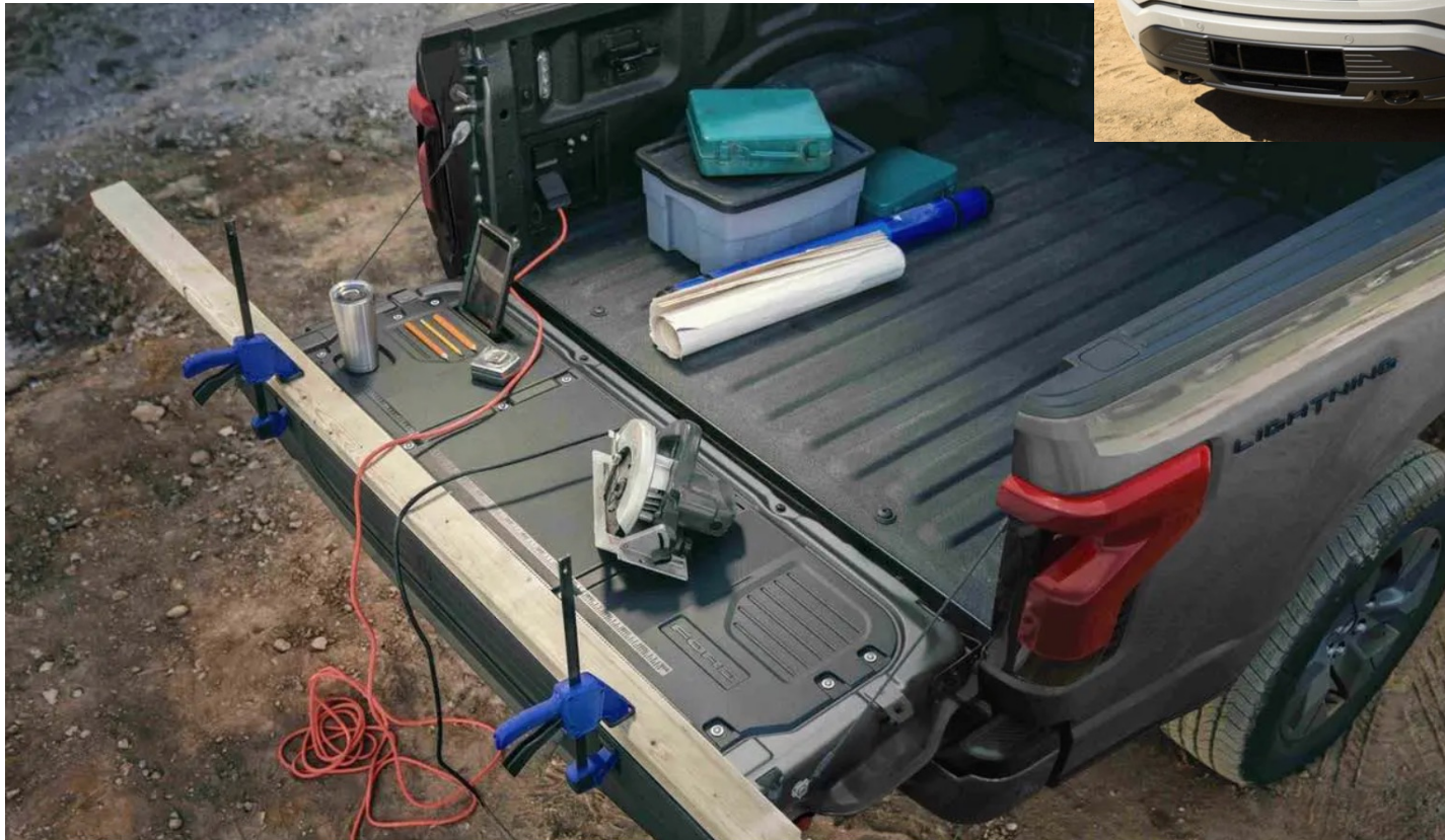
FORD F150 LIGHTNING REAR V2L SOCKET POSITION. IMAGE: FORD.
