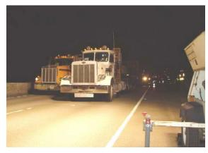
The I-90 load test involved loading trucks and driving them across the bridge to simulate the weight of light rail vehicles
