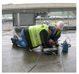
Workers using ground-penetrating radar to locate the steel in the I-90 bridge deck.
